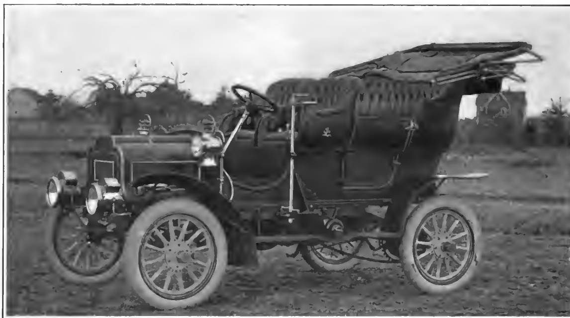
NEW KNOX SIDE ENTRANCE TOURING CAR, WITH TWO-CYLINDER, AIR-COOLED MOTOR AND BONNET FRONT.
